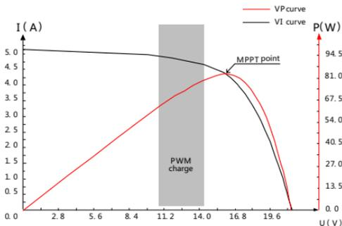
**Fig.1-2 Output Characteristic Curve for Solar Battery**
