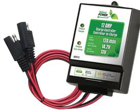
LED light indicates a full battery charge "green" at 14.2 Volts, at this time the charge controller will cut out to prevent overcharging.
