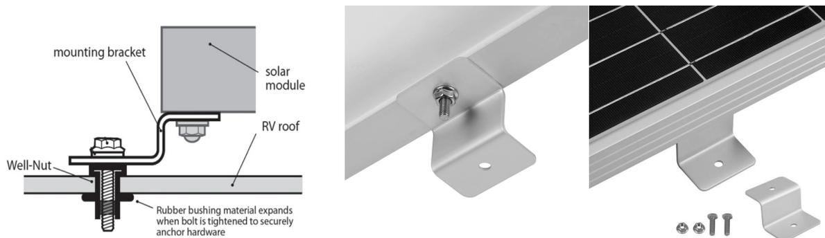
The solar panels can be permanently installed level using the Z-brackets.
