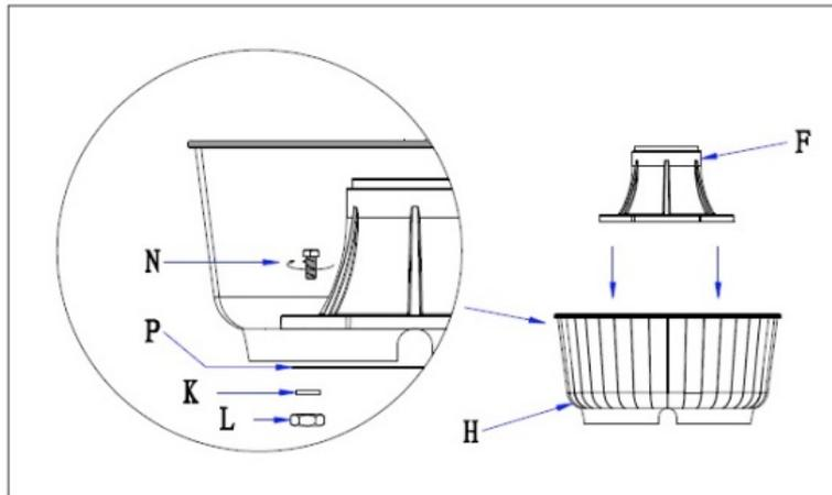
1. (SEE FIGURE 1) Attach lamp post base (F) to Bottom planter base (H) using M10 bolts (N), mounting plate (P), Flat washer (K) and hex Nut (L). Make sure the mounting plate, flat washer and hex nut are secured to the hex bolt on the underside of the bottom of the planter base (H).
