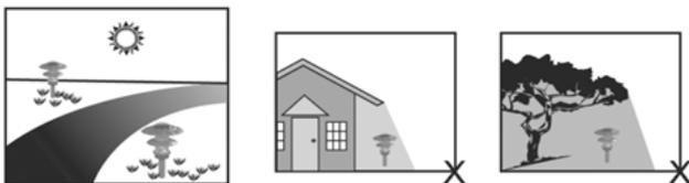
Solar powered lights require sunlight to recharge the internal batteries. For best results, place the solar panel in a position where it will receive direct sunlight, generally free from cover and shade.
