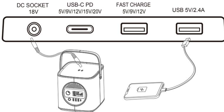
**DC output ports of the solar panel can directly charge a variety of portable electronic devices.**
