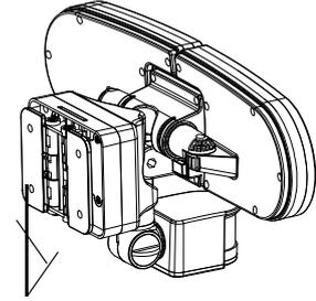
**Note:** The lamp unit should be mounted 6.5-9 feet (2-3 meters), from the ground to ensure motion detection is optimized.
